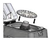
**Note:** 1) Check the tube holder is firmly tightened before running the next program.
